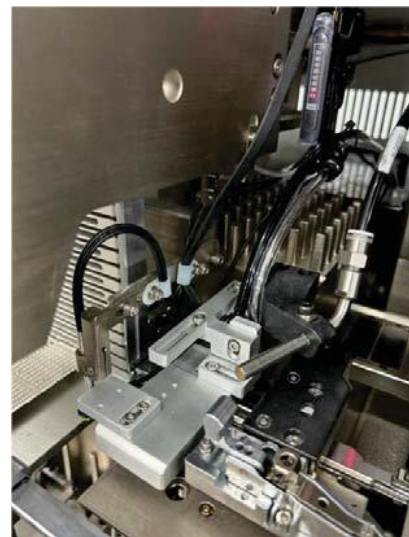
(b) Wire bond machine with integrated blow and suction mechanism.
