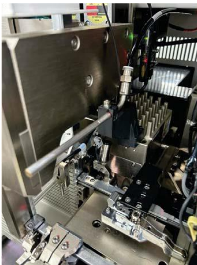
(a) Wire bond machine without cleaning system
